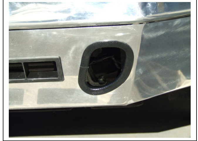
Figure 18: Turn skirt vents upside down to allow maximum airflow to intercooler
