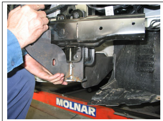
Figure 4: Steel mounting bracket being placed behind bumper support. Passenger's side shown.
