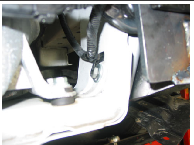
Figure 8: Place bolts through from inside of radiator support.
