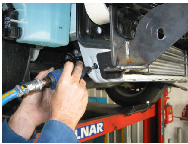
Figure 7: Enlarge hole in radiator support using a die grinder.
